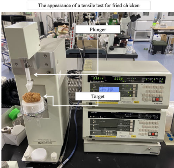
Fig. 7. Representation of the creep meter used in the experiments
