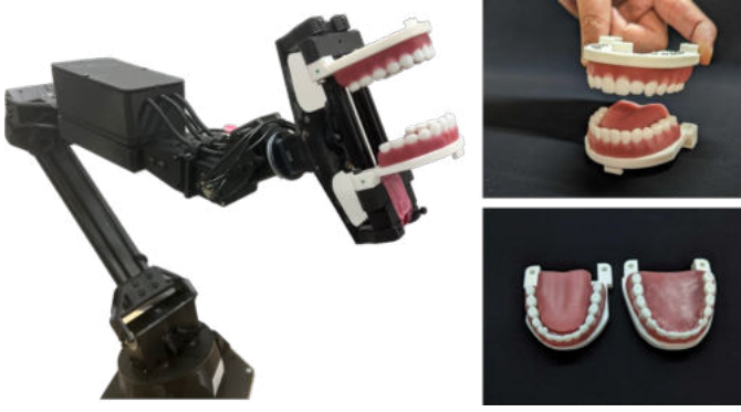
Fig. 2. The appearance of the Gel Biter developed in this study: a model designed to match the dimensions of the human oral structure, with piezoelectric film sensors placed on the upper surface center of the upper jaw, the center of the interior of the tongue, and the lower surface center of the lower jaw
